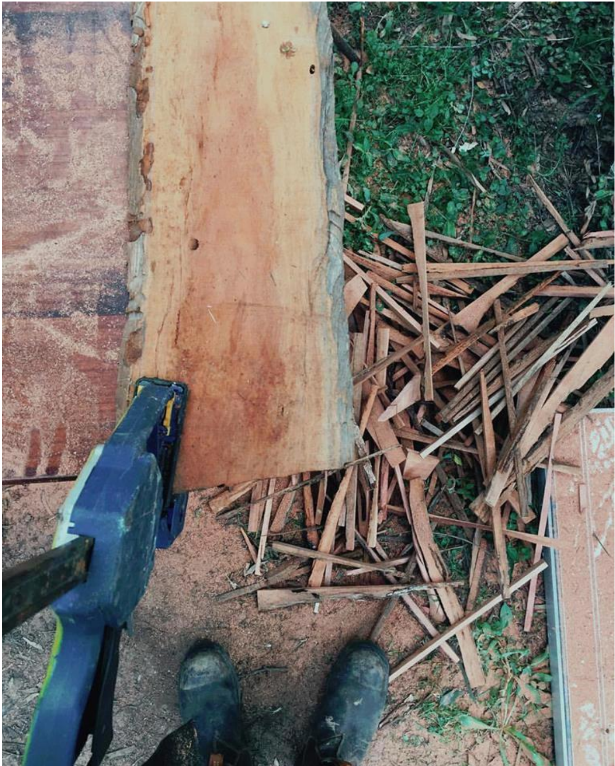
Trimming the live edge of the shingles
